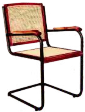
Model No. JOC 411-A Jalaram full arm office chair, seat & back & handle crafted from seasoned teak wood, finished in natural PU coating & cased in special plastic of high tensile strength. Frame from ERW prime quality tube of 16 swg, reinforced at all bends by additional pipe for static and impact load with cushioning effect, powder coated finish after 8 tanks anti rust treatment. Overall Size: H-91.5 x W-53.5 x D-61 (cm)
